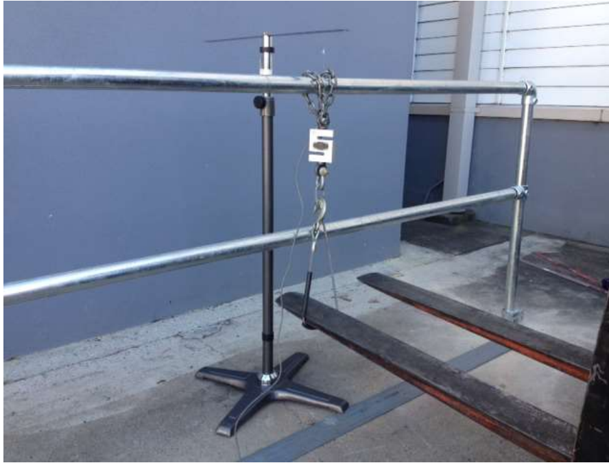
Photo 3: Test # 3 Handrail 2.4mts Top rail
